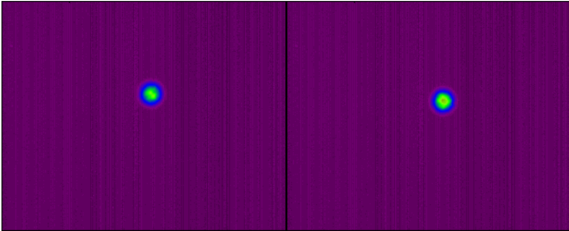
Figure 29. Far-field Images of the Stokes Beam in the 2.5km Fiber with 0 W (left) and 5 W (right) of Pump.
